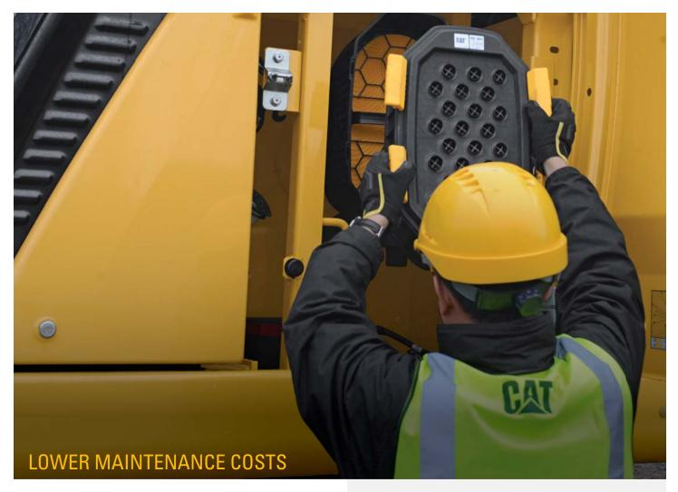
With extended maintenance intervals, you get more done at a lower cost compared to the 336D2. Consolidated filter locations make service faster. Hydraulic, air, and fuel tank filters have increased capacity and longer life.
