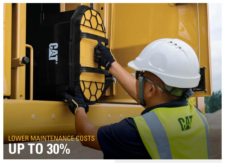
With extended maintenance intervals, you get more done at a lower cost compared to the 349D2 Tier 3 excavator. Consolidated filter locations make service faster. Hydraulic, air, and fuel filters have increased capacity and longer life.
