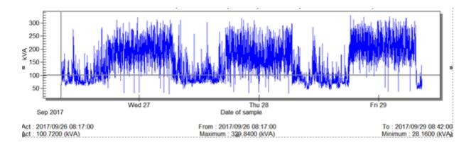
Based on the above information we recommend a 165Kva to provide security of electrical supply during downtimes of your mains electrical supply.
